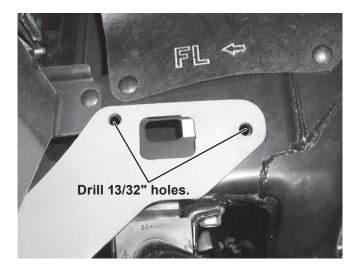
5. Insert two 3/8" x 1-1/4" cap screws with handles and 3/8" flat washers into the inside of the truck frame and out through the rear drilled holes. Attach a 3/8" locknut to each cap screw and hand tighten.
