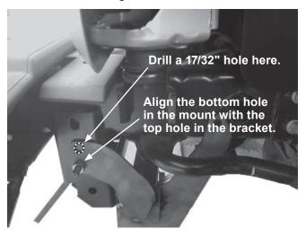
NOTE: Front wheels should be straight ahead for easiest installation.
