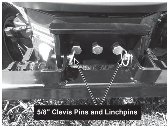
5. Secure the rear arms of the mount beam to the lower lugs of the tractor using two 5/8" clevis pins. Secure each clevis pin with a linchpin. It may be necessary to loosen the front mount plate fasteners and reposition the front mount plate to allow the holes in the rear arms to align with the lower lugs of the tractor. Then tighten the front mount plate fasteners again.
