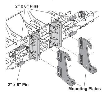
4. Secure each end of each pin with the eight provided 3/8" x 3" cap screws and 3/8" locknuts as shown. Tighten to 30.8 ft-lb (41.8 N·m).
