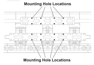
2. Install each attachment plate to the eight indicated holes with 3/4" x 3" cap screws, 3/4" washers, and 3/4" locknuts as shown. The notches in the attachment plates must face the center of the snowplow. Tighten to 269 ft-lb (365 N·m).
