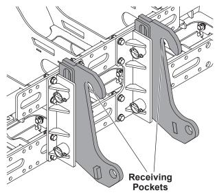
3. Slowly raise the arms on the loader and tilt the loader plate toward the cab until the mount plates are flush with the OEM attachment bracket.
