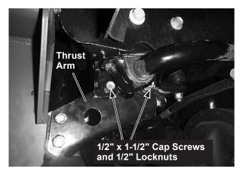
Remove the driver-side and passenger-side stabilizer bar bracket bolts. Save the stabilizer bar bracket bolts for reinstallation if the mount is removed.
