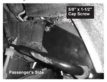
7. On both sides of the vehicle, fasten the thrust arms to the stabilizer bar brackets with two 1/2" x 1-1/2" cap screws and 1/2" locknuts.
