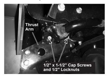
8. Tighten all fasteners according to the torque chart.
