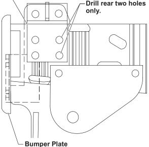
For F-250, F-350, and all other vehicles with swaybar bracket: With the rear of the pushplate fitted snugly to both the side and bottom of the frame, tighten the fasteners running through the swaybar bracket.
