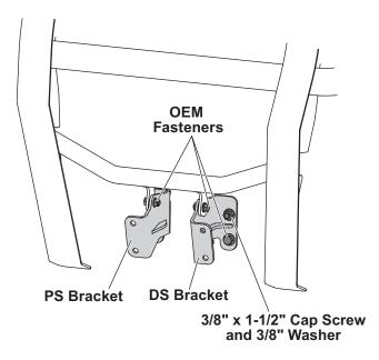
NOTE: The bracket flanges should point outward and the center fastener hole should be on top.
