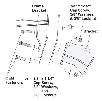
5. For all applications, position the skid plate assembly on the brackets as shown. Secure the skid plate assembly to the brackets with four 3/8" x 1-1/4" cap screws and four 3/8" locknuts.
