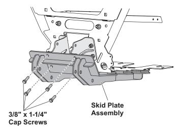
6. Insert a 3/8" x 1-1/4" cap screw with a 3/8" washer through each of the two front skid plate attachment holes. Secure each fastener with a 3/8" washer and 3/8" locknut.
