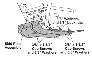
7. Tighten all fasteners according to the torque chart.
