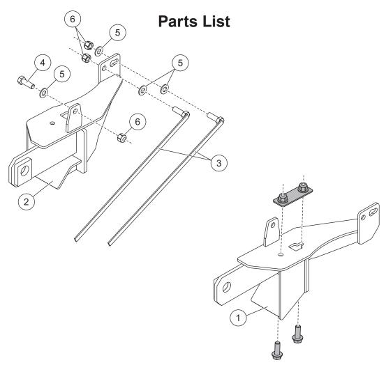
Shaded parts are original vehicle fasteners.
