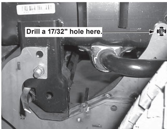
6. Insert a 1/2" x 1-1/2" cap screw with long (18") handle and a 1/2" washer into the front of each frame rail and out through the drilled holes on either side. Attach a locknut and finger tighten.
