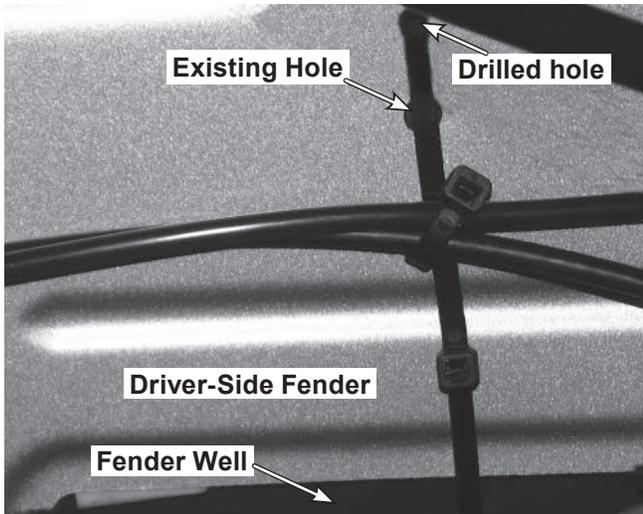
Install the isolation module on the inside of the driver-side fender using the supplied cable ties, reclosable fastener strips and edging material as shown below.
