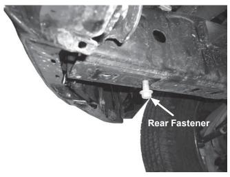
3. Place the passenger-side mount up against the frame. Slide the mount forward around the rear tow hook fastener as shown. Insert the front tow hook fastener up through the mount hole and thread into the nut bar (a clip with 2 nuts attached, original to the vehicle) until the mount lightly touches the bottom surface of the vehicle frame. Do not tighten the fasteners at this time, as the mount must be free to move laterally for the following steps.
