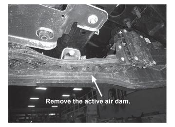
2. Remove the front tow hook fasteners and loosen the rear fasteners. Remove the tow hooks by sliding them forward and then downward. Leave the rear fastener in position as shown.
