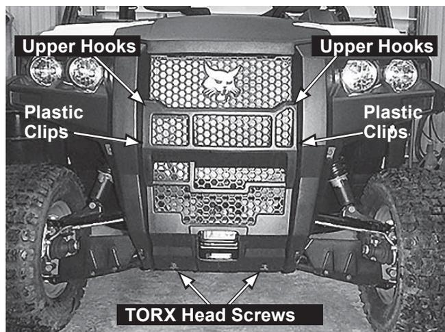
3. Position the skid plate assembly as shown.
