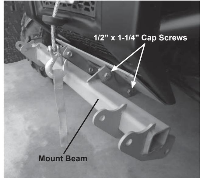
9. Measure the distance between the mount beam rear hole and the ground. If it exceeds 11-1/2", install the accessory Adapter Plates Kit (PN 77555) to ensure optimum plowing performance.
