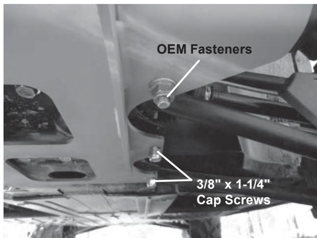
3. To install the driver-side bracket, position the driver-side bracket as shown.
