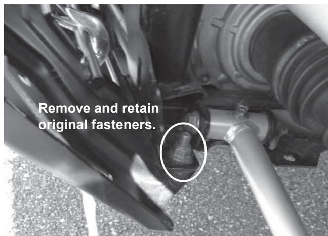
2. Install the mount skid plate assembly as shown. Reuse the OEM fasteners removed in Step 1 in the front holes. Use the supplied 3/8" x 1-1/4" cap screws in the remaining four positions. Fasteners should be finger tight.
