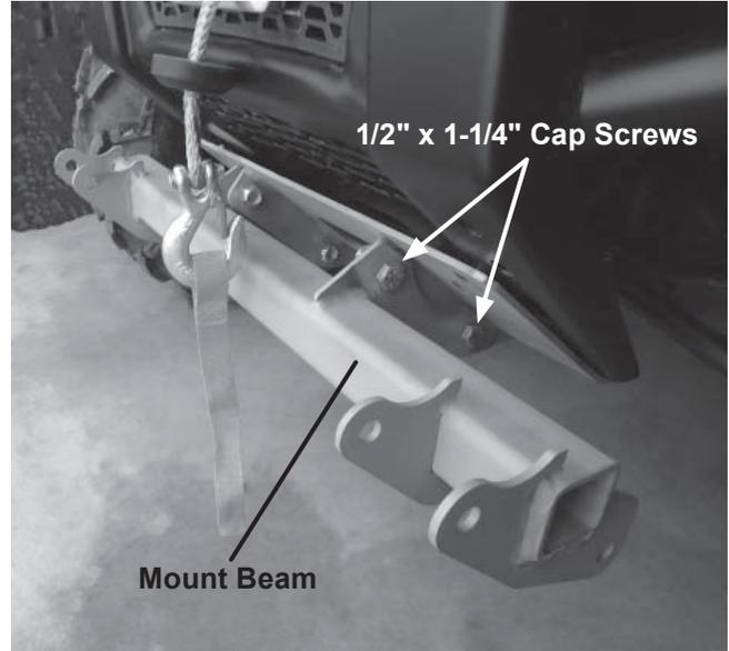
5. Measure the distance between the mount beam rear hole and the ground. If it exceeds 11-1/2", install the accessory Adapter Plates Kit (PN 77555) to ensure optimum plowing performance.
