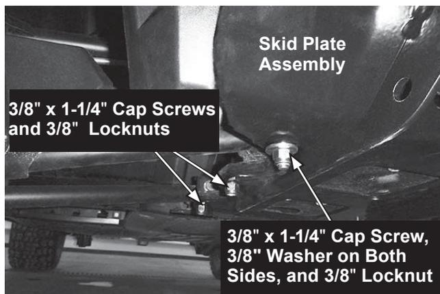
4. To install the passenger-side bracket, position the passenger-side bracket as shown.
