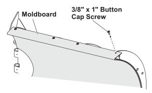
Install the supplied 3/8" x 1-1/2" cap screws and 3/8" flat washers through the blade frame and the moldboard from the bottom up. Install a second 3/8" flat washer and 3/8" locknut to each cap screw and tighten.
