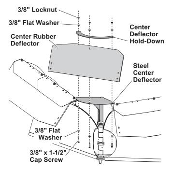
Attach the center rubber deflector to the wing rubber deflectors using the provided 3/8" x 1-1/2" cap screws, 3/8" flat washers, and 3/8" locknuts in the pre-made holes.
