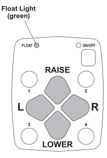
The four diamond-shaped buttons in the center of the control face, when pressed, will result in the blade movements described in the table.
