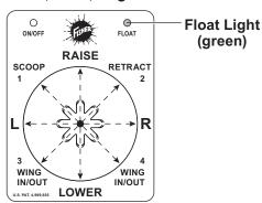
Moving the control lever in straight lines up and down or from side to side on the control body will result in the following blade movements:
