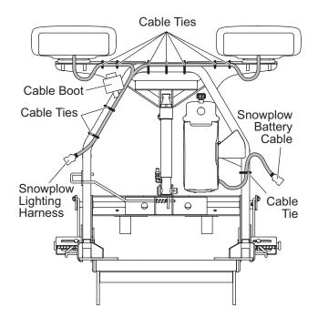
3. Install the cable boot onto the headgear bracket.
