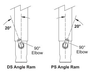
Reattach the base end of the angle ram with a 1" x 4" clevis pin and secure with a 1-1/2" cotter pin. Repeat this process for the second angle ram.
