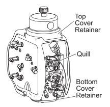
The quill in the valve manifold adjusts the blade drop speed.
