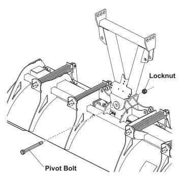
Cut the tie holding the angle rams to the A-frame. Remove the protective caps on the angle rams. Swing the A-frame to one side so that the holes in the rod end of the angle ram and the blade are aligned. 4. Install a 1" x 4-3/4" clevis pin from the top down. Swing the A-frame to the other side and secure the second angle ram in the same manner. Secure the angle rams by installing 1/4" x 1-1/2" cotter pins in the two rod-end clevis pins.
