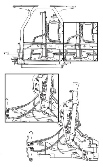
4. Using a wrench to hold the hose end in position, tighten all hose fittings 1/8–1/4 turn past finger tight.
