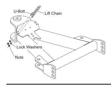
Place a U-bolt on the extension spring. Attach a 3/8" nut on each side of the U-bolt. Insert the U-bolt through the mounting tab on the A-frame. Place lock washers and 3/8" nuts on the U-bolt and tighten.
