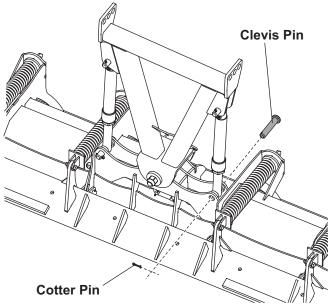
5. Remove the 1" x 4" clevis pin from the base end of one of the angle rams and install the fitting as shown.
