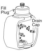
With wing and lift rams fully retracted, fill the reservoir with FISHER<sup>®</sup> EZ Flow Hydraulic Fluid to -40°F (-40°C), or other fluid conforming to Military
