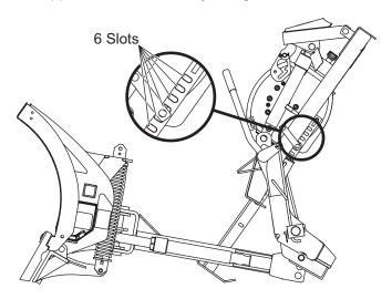
A-frame and push assembly. Attach the jack handle to the jack with a 3/8" lock washer and nut.
