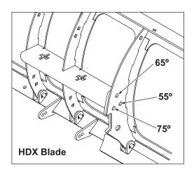
5. Align the back drag edges against the front of the blade base angle, matching up the holes that correspond to the blade attack angle.
