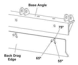
6. Install the back drag edges and cutting edge to the base angle using the supplied 2-1/2" carriage bolts and locknuts.
