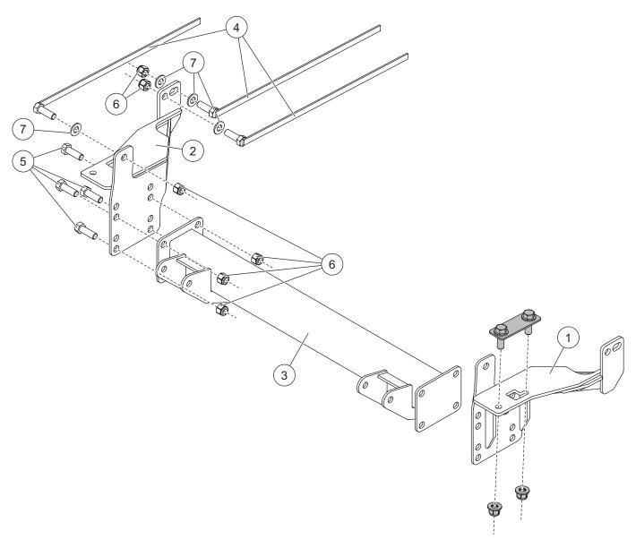
Shaded parts are original vehicle fasteners.
