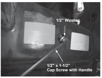
8. Secure the other side of the frame rail with a 1/2" washer and 1/2" locknut as shown. Hand tighten the fasteners so that the mount tab comes just into contact with the frame rail. Do not fully tighten at this time. Repeat Steps 7 and 8 on the driver's side of the frame rail.
