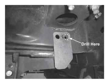
7. Attach a 1/2" washer to each of two 1/2" x 1-1/2" cap screws with handles and insert them into the frame rail through the opening shown and then through the mount holes. Start with the front mount hole to ensure that the rear fastener handle will not block access.
