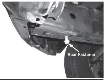
3. Place the passenger-side mount up against the frame. Slide the mount forward around the rear tow hook fastener as shown. Insert the front tow hook fastener up through the mount hole and thread into the nut bar (a clip with two nuts attached, original to the vehicle) until the mount lightly touches the bottom surface of the vehicle frame. Do not tighten the fasteners at this time, as the mount must be free to move laterally for the following steps.
