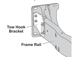
3. Install the mount by holding the front portion of mount in place and securing with the previously removed bumper bracket bolt assembly. Clamp the rear portion of the mount into position on truck frame, making sure the mount is tight against the bottom of the frame.
