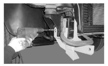
Pull up and forward on the bottom tab of the frame spacer, allowing enough room to install the handled cap screws. Insert three handled 1/2" x 1-1/2" cap screws and two 1/2" hardened flat washers past the opening in the front frame spacer and into the truck frame. (Do not put a washer on the cap screw that goes through the bottom of the frame.) Fasten with three 1/2" locknuts. Hand tighten fasteners. Bend or cut off the handles on the cap screws to prevent contact with the bumper bracket.
