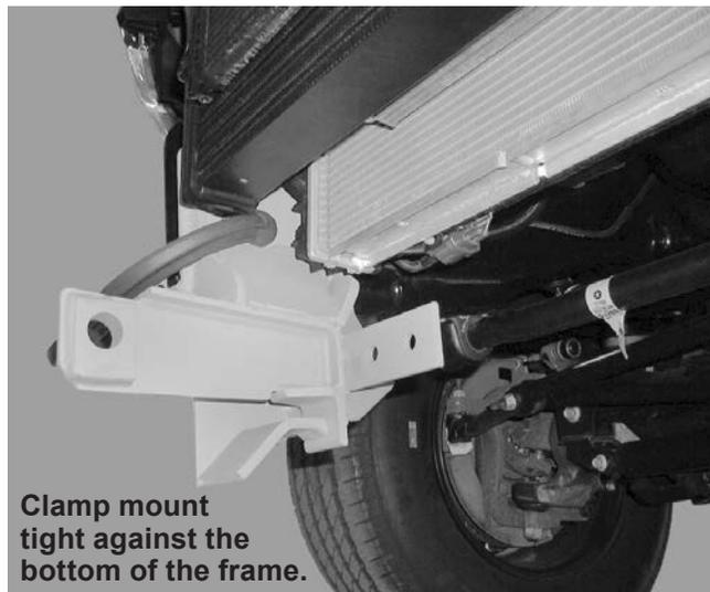
Vehicles equipped with tow hooks will need the tow hooks and tow hook brackets removed. These cannot be reinstalled with snowplow mount. Retain tow hooks, brackets, and fasteners for reinstallation if snowplow is removed.
