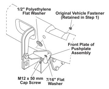
11. Tighten fasteners according to the torque chart, in the order indicated below.
