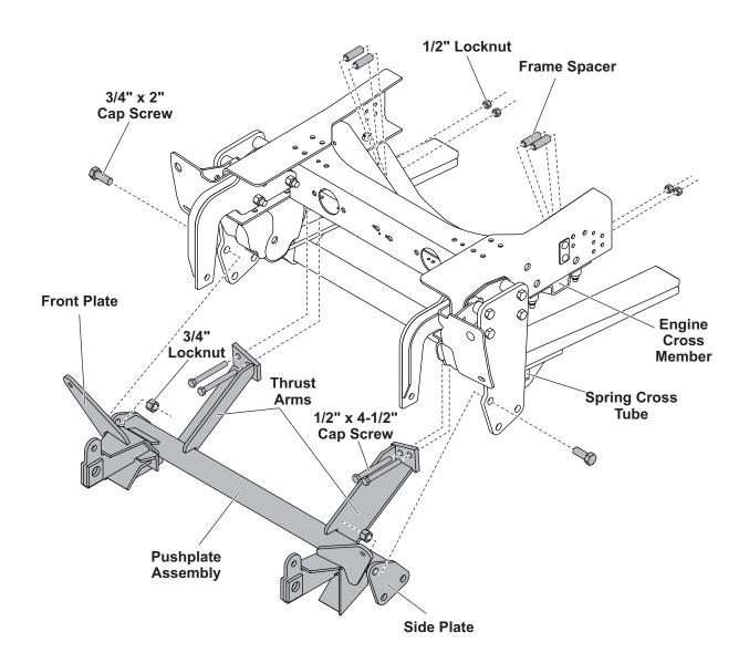
Bumper not shown for clarity. Do not remove bumper during installation.
