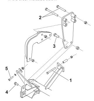
NOTE: After five to ten hours of snowplow usage, retorque all pushplate assembly fasteners.
