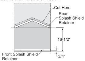
3. Position the splash shield on the vehicle so that the tapered end with three holes is toward the rear of the truck and the shield is on top of the cross bar. Using the vehicle splash pan fasteners, place two fasteners up through the front splash shield retainer bar, rubber shield, and into the original splash pan fastener holes at the front. Place three fasteners up through the rear splash shield retainer bar, rubber shield, and into the original splash pan fastener holes toward the rear.
