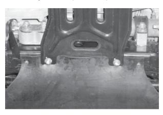
If the vehicle is not equipped with a transaxle skid plate, align the holes in the rear splash shield retainer and the tapered end of the splash shield with those in the vehicle frame cross member. Install two M6 x 1.00 cap screws and flat washers (supplied with the mount) through the rear splash shield retainer and splash shield and into the cross member. Do not overtighten.
