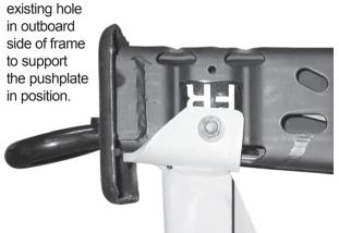
Install, but do not tighten, the remaining two tow hook fasteners.
