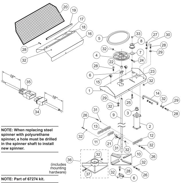
This Parts List is for FISHER<sup>®</sup> SPEED-CASTER Tailgate Spreaders with serial numbers beginning with 115297 and higher.
