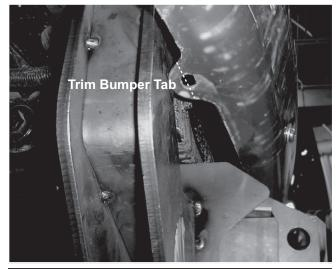
NOTE: After five to ten hours of snowplow usage, retorque all pushplate assembly fasteners.
