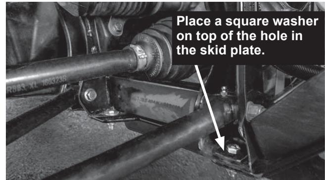
2. Position the skid pan assembly against the underside of the UTV and align its four outer slotted holes with the holes in the bottom of the UTV.
