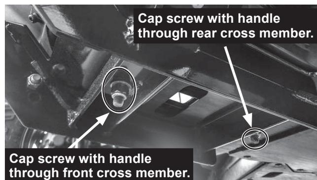
Bend or trim handles after installation to avoid interference with vehicle components.
