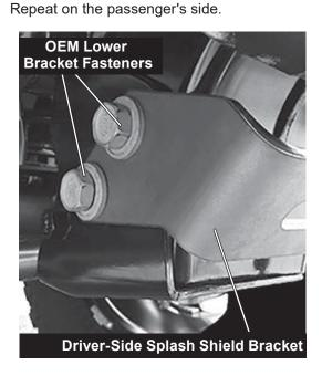
14. Reinstall the bumper and trim the splash shield as shown. Secure the splash shield to the lower splash shield brackets using the original fasteners. Secure the splash shield to the upper splash shield brackets using the 3/8" fasteners provided.
