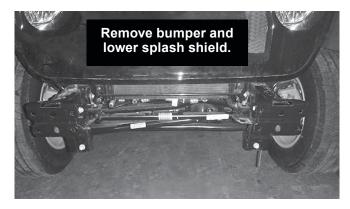
**For Gladiator models:** Remove the upper and lower splash shield brackets, if so equipped. Save the fasteners for reinstallation.
