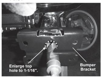
9. Insert a 1/2" x 1-1/4" flanged cap screw with 18" handle into the frame through the enlarged bumper bracket hole. Guide the flanged cap screw out through the rear hole of the mount plate.
