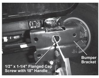
Secure the cap screw with a 1/2" locknut. Hand tighten the locknut.
