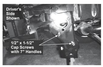
3. Place the driver-side mount plate against the underride structure, allowing the fasteners to protrude through the holes in the mount plate. Secure the mount plate using two 1/2" locknuts. Tighten the locknuts, but do not fully tighten them at this time.
