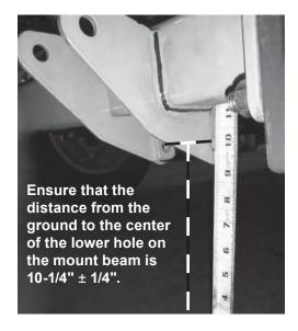
Check that the mount is level and make adjustments as necessary. Secure the mount by installing a 1/2" locknut on each 2-1/2" cap screw. Hand tighten the locknuts.
