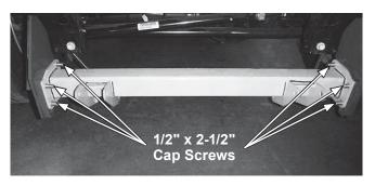
Use the set of holes that positions the mount at 10-1/4" +/- 1/4" from the ground when measured as shown.
