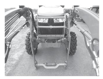
Remove the brush guard assembly (if equipped) by removing the fasteners from the brush guard arms. Save the fasteners for re-installation if the snowplow mount is removed.
