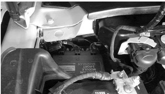
Isolation module, after installation.
