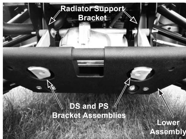
Secure the bracket assembly to the radiator support bracket using 3/8" x 2-1/2" cap screws. Place two 3/8" washers on each cap screw—one on each side of the bracket assembly—and fasten with 3/8" locknuts. Hand tighten.
