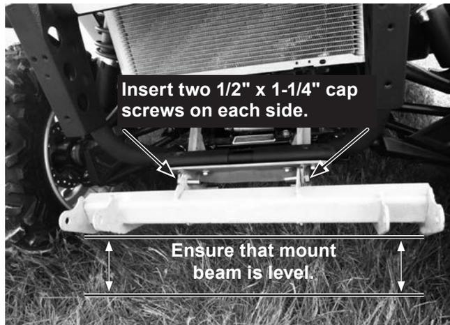
12. Tighten all fasteners according to the torque chart.
