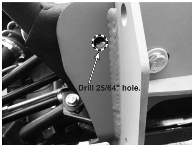
8. Insert a 3/8" x 1-1/4" cap screw up through each hole drilled in Step 7. Secure with a 3/8" washer and 3/8" locknut. Tighten according to the torque chart.
