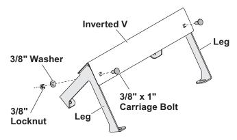
Inverted V for 0.35 yd3 hopper spreader shown.
