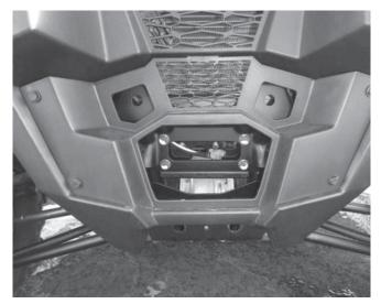
2. Align the innermost holes on the front of the skid plate assembly with the holes in the front of the UTV as shown below.
