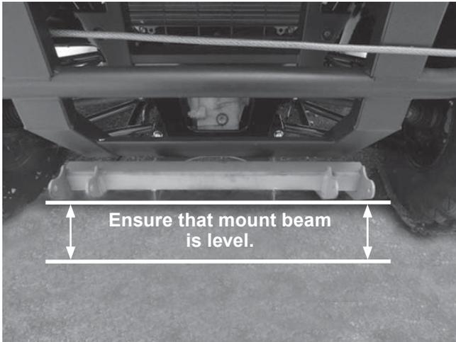
12. The distance from the ground to the lowest receiving hole on the mount beam should be approximately 10-1/4". Suspension adjustment may be necessary to achieve the proper ground clearance.
