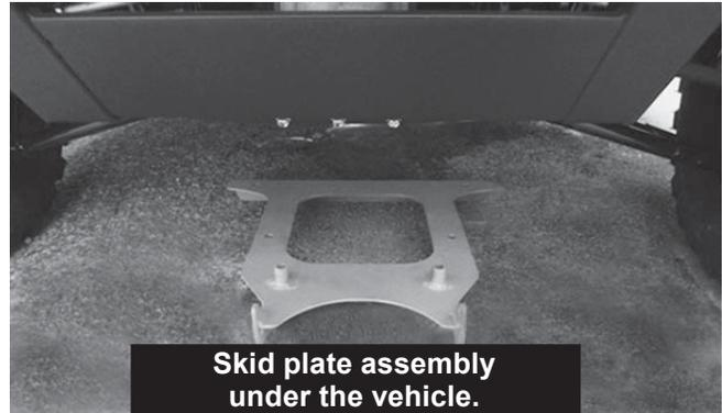
2. With the help of a second person, hold the skid plate assembly against the bottom of the frame. Center the skid plate from left to right. Be sure that the tail of the skid plate is between the two frame uprights. The passenger's side is shown in the picture below.
