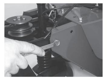
2. Remove the cap screws on both sides that hold the wheel drive housing to the brush drive frame. Pull the brush drive frame forward keeping the frame-member as level as possible and keeping the frame from scraping the cover. DO NOT REUSE THE REMOVED HARDWARE.
