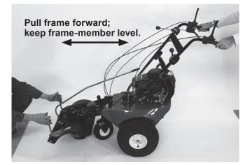
3. Loosely preassemble the brushing subassembly to the axle drive housing with cap screws and washers. Begin at the front.
