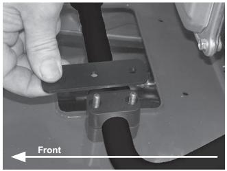
5. Put M6 locknut and washer on the stud.
