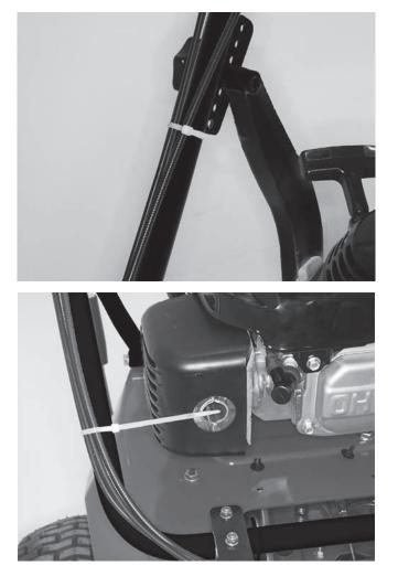
The ties here must form a loop. Do not tighten completely. The cable must be able to move when the handle is folded.
