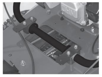
7. Using a 10 mm wrench, attach throttle lever with M6 x 65 mm cap screw, washer, and locknut.
