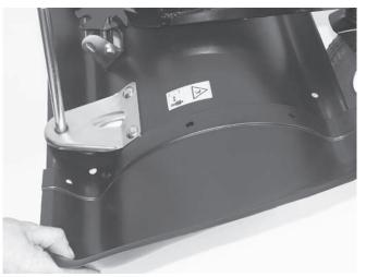
3. Push the cap screws through from above. Push the washers on from below, and screw on the nuts. Tighten with a 13 mm wrench.
