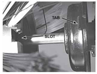
7. Put the left brush on. Make sure the brush is locked onto center cap-gear.
