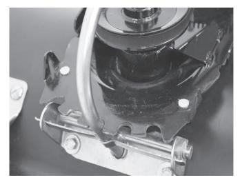
13. Set the brush at an angle. Slip the cover over the belt area and back so the snap Nuts can be seen through the holes in the cover.
