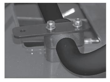
6. Tighten the nuts so the handlebars will still move, but not fall.
