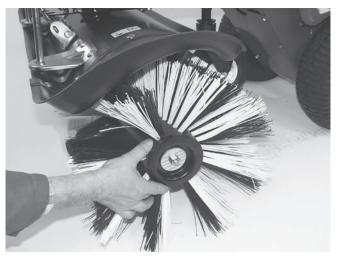
5. Put the axle with the cap, washer, and brush through drive source (centered underneath the brush cover).
