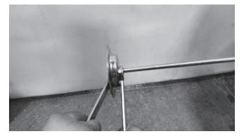
4. Put the axle with the cap, washer and right brush through the drive source (centered underneath the brush cover).
