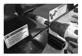
4. De-burr the edge of the hole and insert the supplied break-thru plug.
