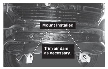
NOTE: After five to ten hours of snowplow usage, retorque all mount assembly fasteners.
