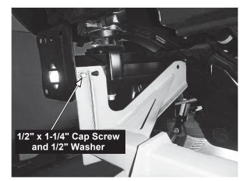
6. Ensure that the mount stops are still contacting the frame. Using the rear mount holes as guides, drill 33/64" holes through the frame.
