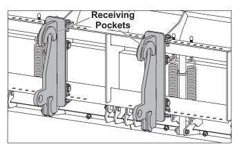
3. Slowly raise the arms on the loader and tilt the loader plate toward the cab until the snowplow mount plates are flush with the JRB 416 attachment plate.
