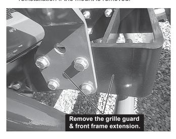
3. Position the left-hand mount plate against the left frame rail of the tractor. Install a 1/2" x 2" cap screw through the rear hole of the mount plate. Secure the cap screw with a 1/2" washer and 1/2" locknut. Tighten, but do not torque the fastener at this time.
