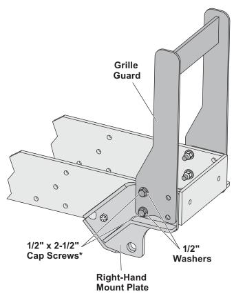
6. On the left side of the tractor, place a bracket against the inside of the left-hand frame rail and front plate. Place a 1/2" washer on each of two 1/2" x 2-1/2" cap screws\*. Install the cap screws through the forward holes of the grille guard/mount plate/frame and out through the bracket. Secure the cap screws with 1/2" washers and 1/2" locknuts. Hand tighten.
