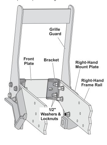
8. Place the front mount plate against the front frame plate of the tractor. Install two 1/2" x 2" cap screws through the holes of the mount plate and out through the brackets.
