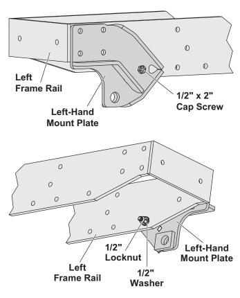
4. Position the grille guard over the left-hand mount plate. Place a 1/2" washer on each of two 1/2" x 2-1/2" cap screws\*. Align the holes in the grille guard, mount plate, and tractor frame. Install the cap screws with washers through the rearmost holes of the grille guard/mount plate/frame. Secure the fasteners with 1/2" washers and 1/2" locknuts. Hand tighten.
