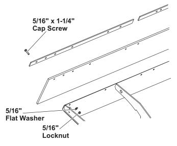
3. On 6' 8" blades, the deflector extends beyond the ends of the blade. Trim excess length from both ends of deflector and retainer bars as shown.
