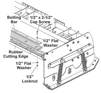
3. Adjust the position of the rubber cutting edge so that it extends approximately 1" beyond the bottom of the blade base angle. Tighten all the fasteners until the rubber starts to bulge.
