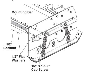
2. Lay the rubber cutting edge and bolting bar onto the mounting bar. Align the holes and insert the 1/2" x 2-1/2" cap screws, 1/2" washers, and 1/2" locknuts.
