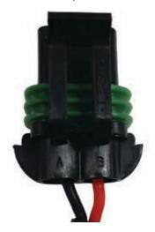
5. Insert terminal extraction tool or paperclip into the connector body as shown to a depth of about 5/16" to release the terminal lock on the red wire.
