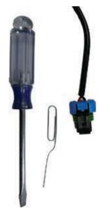
3. Gently pry secondary lock away from each side of connector body and set it aside for reuse.
