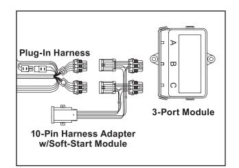
5. Mount the soft-start module in an area that receives good airflow, such as the cavity between the grille and the radiator.
