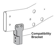
Remove the nuts from the bumper fastener assembly on both sides of the vehicle. For both driver-side and passenger-side mounts, align the forward mount holes with the protruding cap screws and guide the mounts onto the respective fastener assembly. Loosely fasten by reinstalling the original nuts.
