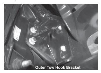
2. Remove the compatibility brackets from the frame, if so equipped (see illustration below). Save the brackets and hardware for the vehicle owner.
