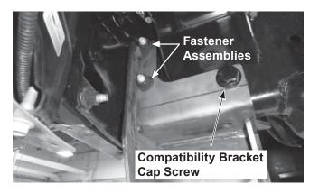
If the vehicle was equipped with compatibility brackets, reinstall one of the original bracket cap screws through the rear hole of each mount and the existing hole in the vehicle frame. Secure with the original nut.
