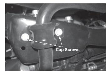
Position a stabilizer bracket between the bottom of the frame rail and the stabilizer bar retainer for both sides, facing inward as shown below.
