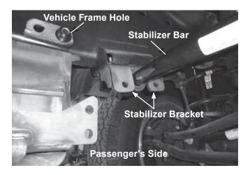
Loosely fasten with the M10 cap screws provided.
