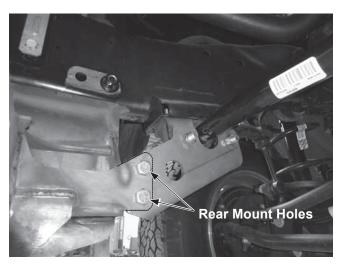
Thrust arms are interchangeable and can install on either side of the vehicle. There is no left or right side-specific part.
