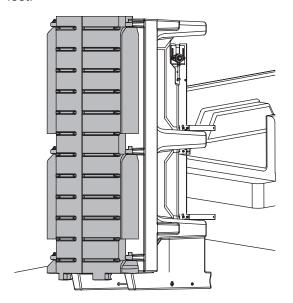
7. **Do not leave an unsecured spreader standing on its feet.** Lower the spreader so it is resting on its 6 legs and place spacers under the legs so the feet at the rear of the spreader are off the ground.
