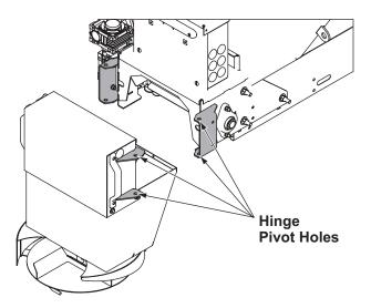
The chute can pivot on either pin to provide access to the feed area of the hopper. An interlock prevents the feed system from running if the chute is rotated to either side or removed.
