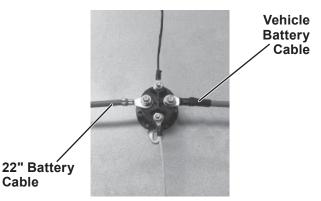
11. Connect the spreader cable (PN 66425) to the vehicle cable (PN 66242).
