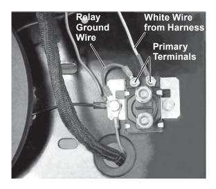
3. Connect the red starter cable (PN 22511K) from the starter to one of the large secondary terminals on the starter relay.
