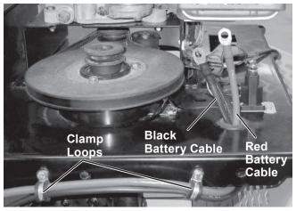
Connect the charge wire (Honda and Briggs & Stratton) or alternator wire (Tecumseh) and the red battery cable to the unused secondary terminal of the starter relay.
