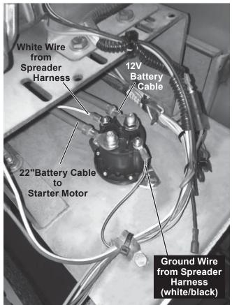
7. Verify the black wire from the spreader harness to the engine shut-off circuit is connected.
