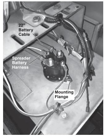
2. Install the red battery cable (PN 66246) to one of the large secondary terminals of the starter relay and to the POSITIVE (+) battery terminal.
