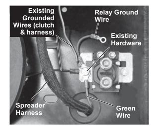
2. Connect the white wire from the spreader harness to one of the primary (small) terminals of the starter relay and connect the relay ground wire to the other small primary terminal on the relay.
