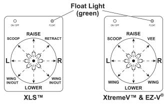
Moving the control lever in straight lines up and down or from side to side on the control body will result in the following blade movements:
