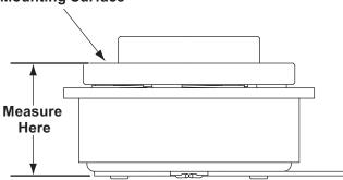
If the new clutch is taller than the old, use the provided 3/16" spacer plates to make up the difference in height. The combined height of the spacer plates and the old clutch should be within 3/32" of the new clutch.
