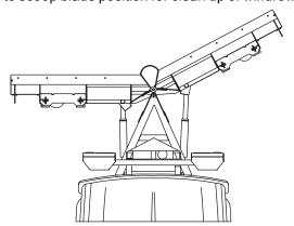
NOTE: For best road clearance during transport, place the blade halfway between the straight and vee positions. The scoop position is NOT RECOMMENDED during transport.
